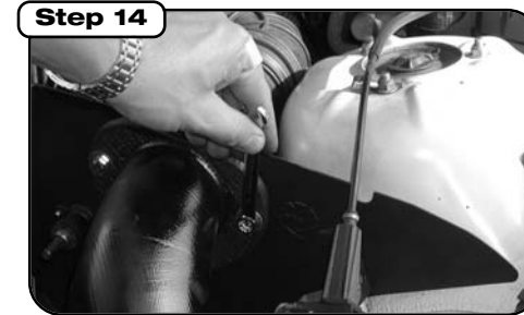
Use the three longest M6 bolts and washers provided to bolt the tube flange to the housing.
