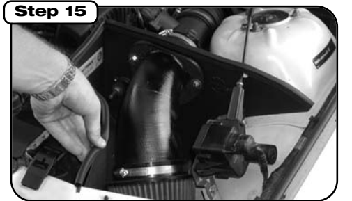
Install trim seal. Make sure all clamps are tight and that all electrical components are secure. Check and retighten connections and filter after a few hours of operation.
