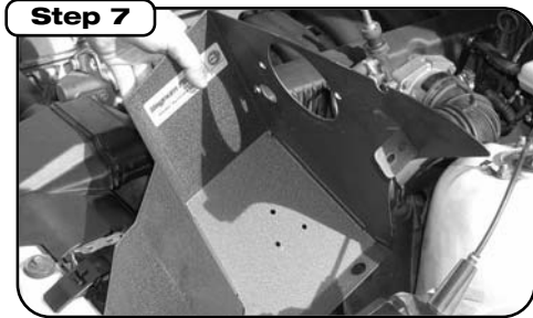
Install the aFe housing into the vehicle.
