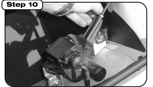
Place cruise control module back in location and use M6 bolts, screws, washers and lock washers supplied with kit.
