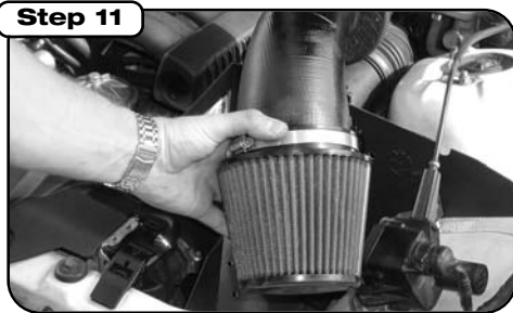
With filter attached to tube but not tightened, slide filter down into fenderwell area and insert mass air sensor into tube.
