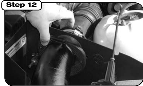
Make sure tube is pressed onto the mass sensor.
